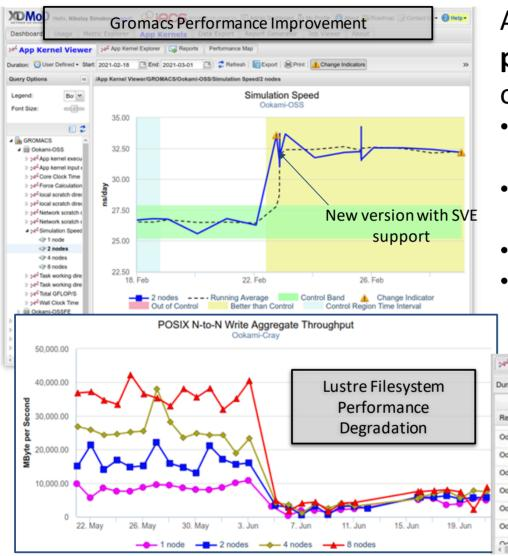
Application kernels module allows **continuous performance monitoring** by periodic execution of applications and benchmarks.
